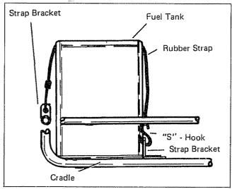
1. Set Fuel Tank into place on alternator cradle. Pass rubber strap UNDER fuel tank lifting handles and hook into both strap brackets.
